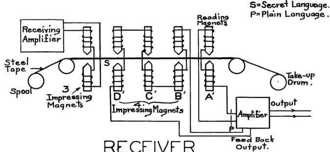
SYSTEM AND MEANS FOR ENCIPHERING AND DECIPHERING MAGNETICALLY-RECORDED SIGNALS.
