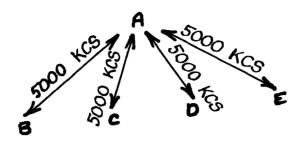
A sends to B, C, D and E on 5000 KCS. B, C, D and E send to A on 5000 KCS.
