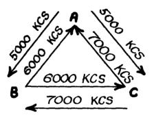
A sends to B and C on 5000 KCS B sends to A and C on 6000 KCS C sends to A and B on 7000 KCS
