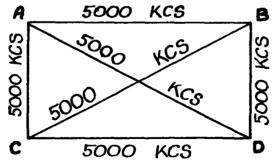
h. <u>Complex Star (CX-STAR)</u> - A net in which the control is assigned one frequency while the outstations are assigned other frequencies. This is similar to the Star in form, but several frequencies are employed instead of one. Often part of the outstations will operate on one frequency while the remainder operate on another.
